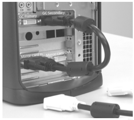
Figure 8. Short DVI cable installed.
