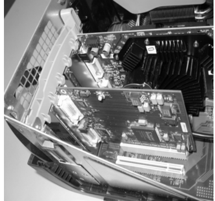
Figure 7. Mirror-flip PCI card installed.
