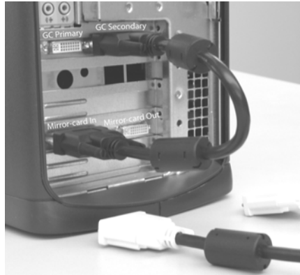
Short DVI cable installed.
