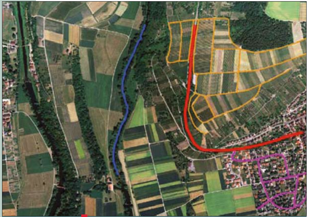
The IMAGINE Easytrace module makes it quick and easy to capture linear features such as road and river centerlines.
