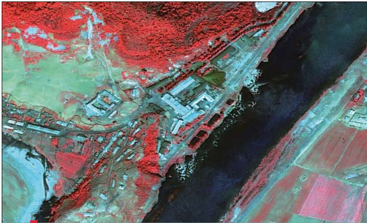
Results of applying the new High Pass Filter resolution merge technique to merge a QuickBird multispectral scene with the corresponding pan scene (co-registered using the new IMAGINE AutoSync module) and produce a 0.61m color image. This new technique retains the spectral (color) information, while maximizing the spatial content, much more effectively than previous algorithms permitted.
