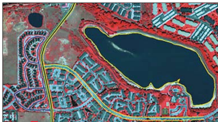
The power of IMAGINE Easytrace also enables the creation of ribbon features (both edges simultaneously) and the tracing of polygon boundaries.
